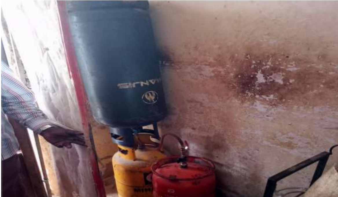
Figure 31: 38kg gas cylinders from Manjis being decanted to 6kg gas cylinders from Lake and Oryx
